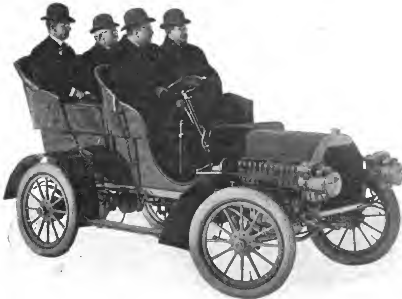
POPE-TRIBUNE SIDE-ENTRANCE TOURING CAR WITH VERTICAL TWIN-CYLINDER MOTOR. 12
